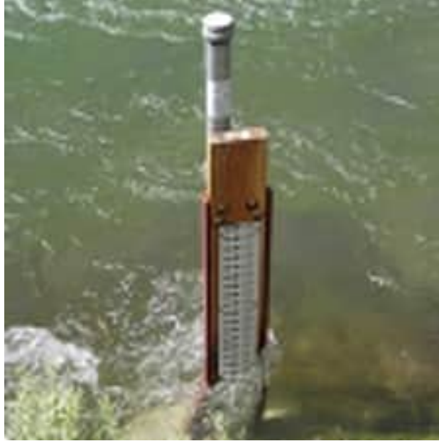
Figure 6 – Simple Stilling Well and Staff Gage Setup
